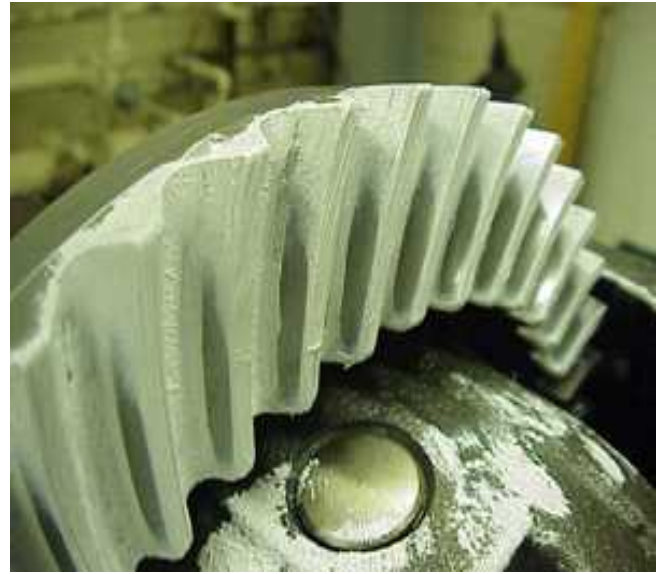
After Test Contact Pattern
