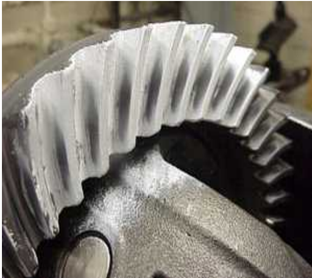
Before Test Contact Pattern
