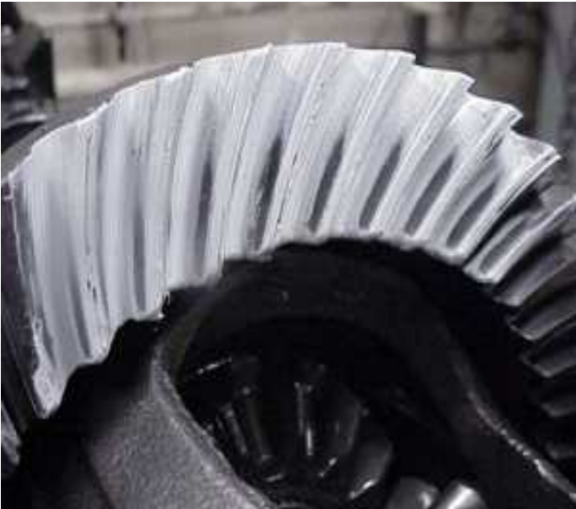
After Test Contact Pattern
