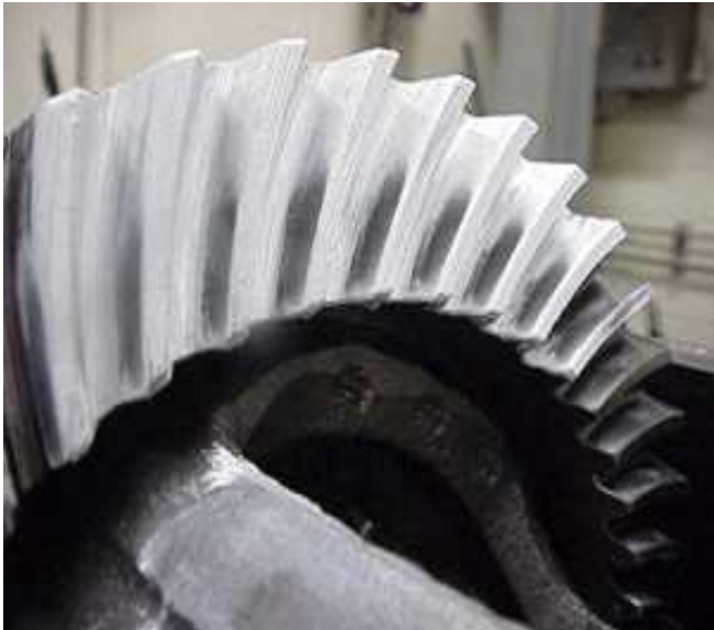
Before Test Contact Pattern
