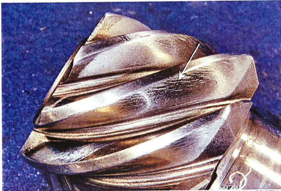
FIGURE 4: SWRI SAMPLE TYPICAL PINION GEAR CONTACT PATTERN ON TOOTH COAST SIDE. THE PATTERN IS MORE LIGHTLY POLISHED WITH SOME SCORING ON THE UPPER FLANK OF THE CENTRAL TOOTH REGION.
