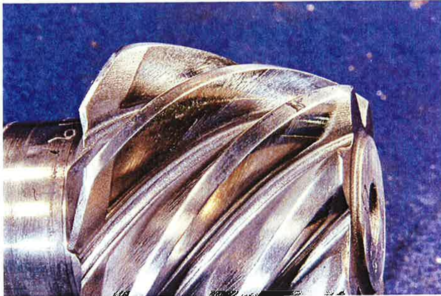
FIGURE 2: SWRI SAMPLE TYPICAL PINION GEAR CONTACT PATTERN ON TOOTH DRIVE SIDE. THE PATTERN HAS A DARKER REGION WITH POLISH AND RIDGING AT THE HEEL END, WHICH TRANSITIONS TO REGION OF LIGHTER POLISH AND RIDGING AT THE TOE END.
