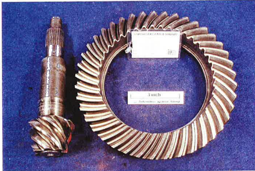
FIGURE 1: SWRI SAMPLE HYPOID DRIVE GEAR SET AS RECEIVED.
