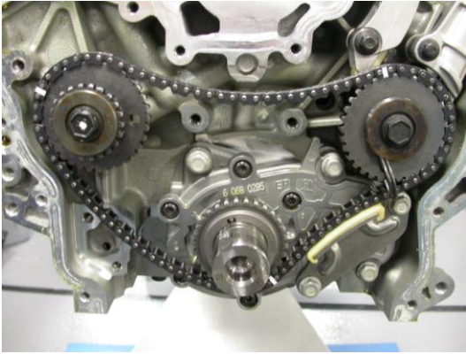
View of primary chain installed.
