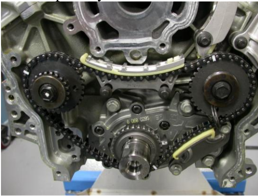
Install primary chain guides.
