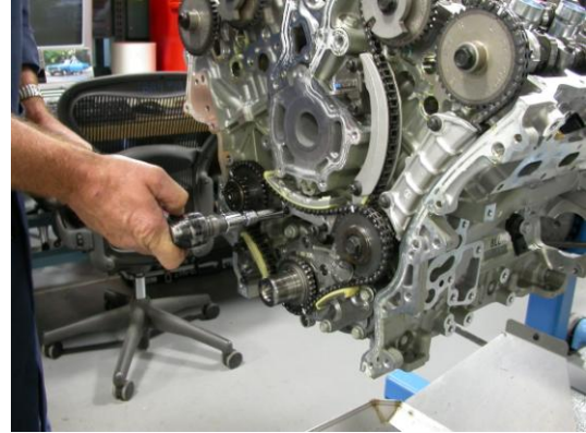
Torque right side idler gear to 58 +/- 7Nm.
