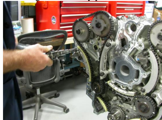
Torque tensioner and chain guides to 23 +/- 3Nm.
