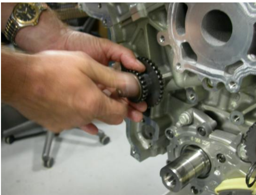
Install right side idler gear and torque to 58 +/- 7Nm.
