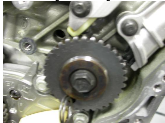
Make sure left side idler gear still has grenade pin holding chain assembly in proper position.
