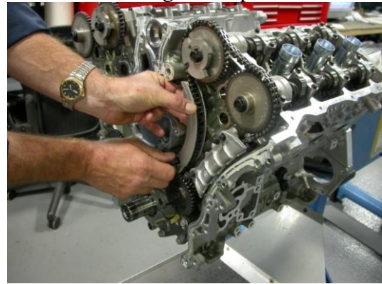
Install left side chain guides.
