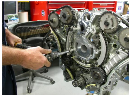
Torque tensioner and chain guides to 23 +/- 3Nm.
