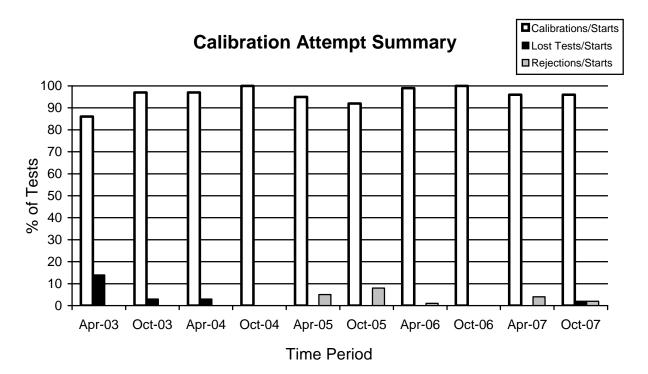
The calibration per start rate remained the same, the lost test per start rate has increased, and the rejected per start rate has decreased when compared to the last report period.
