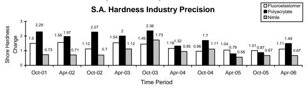
Percent volume industry precision estimates for elastomer materials, for the last ten report periods are shown below. Precision for polyacrylate, fluoroelastomer, and nitrile elastomers have degraded slightly with respect to the previous period. Precision for all three elastomers compares well with respect to historical levels.
