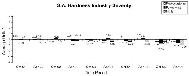
Percent volume industry mean delta/s bar charts for the last ten report periods, for each elastomer material are shown below. Percent volume for the polyacrylate and nitrile materials trended mild and the fluoroelastomer material trended severe of target for this report period.
