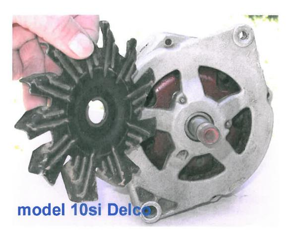
In the above photo, the pulley and cooling fan has been removed from the front of a model 10SI alternator. The factory built this model with a maximum of 63amp output rating. In the photo below, we will see the next generation alternator, a model 12SI, which is equipped with a high performance fan.
