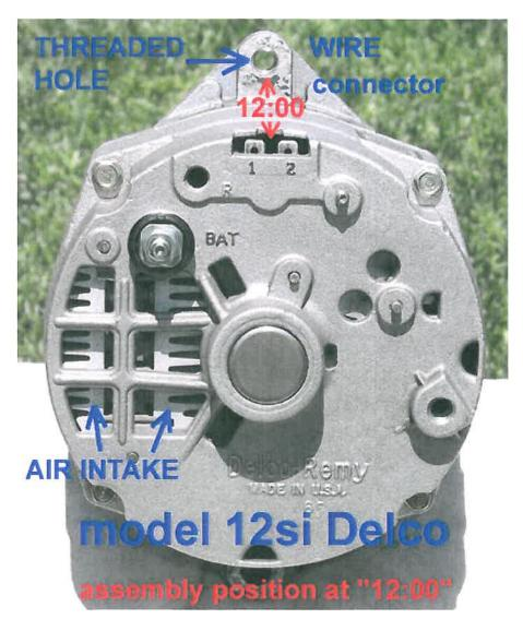
The photo above shows a model 12SI Delco alternator, viewed from the rear. Notice the increased air intake area with this 12SI, as compared to the 10SI. When viewed from the rear, the greater air intake area is the most distinguishing visible feature of the 12SI. (The rear view of a 10SI was shown in a previous photo, above.)
