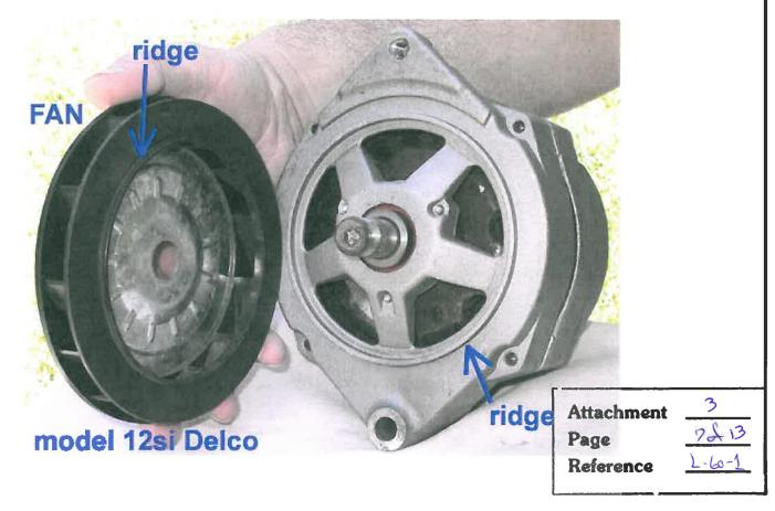
And in the photo above, the pulley and cooling fan has been removed from a "stock," model 12SI, Delco Remy built alternator. Compared to the fan on the 10SI, the 12SI fan is certainly a high performance design.
