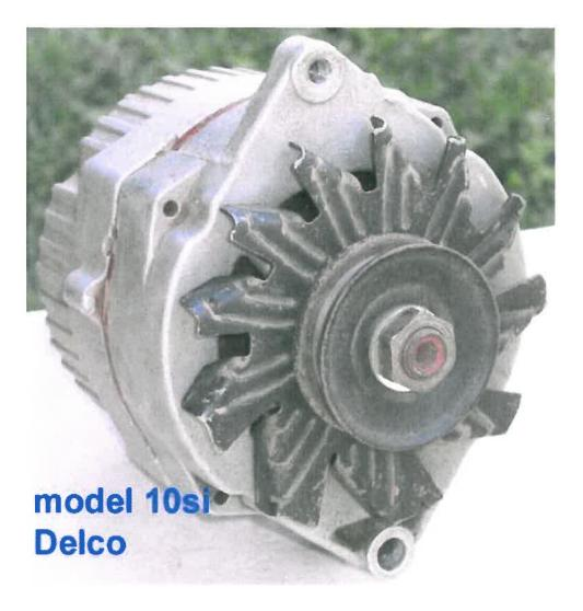
The photo above shows a typical, used, model 10SI, Delco Remy built alternator.
