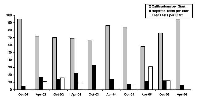
The calibration per start has increased this report period when compared to the previous period. The lost test per start rate and the rejected test per start rate has decreased this report period when compared to the previous period
