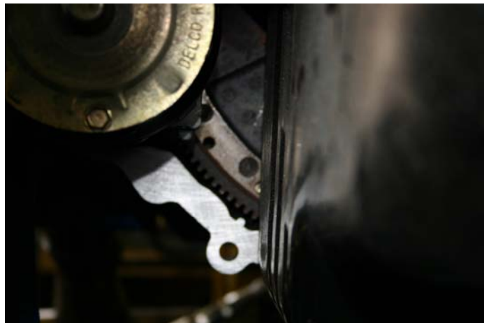
Flywheel Location Remove Starter to Access Labs Code Flywheel through Hole
