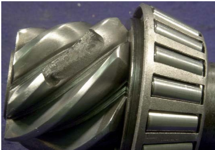
FIGURE 4: PINION SHOWING TOOTH FAILURE.
