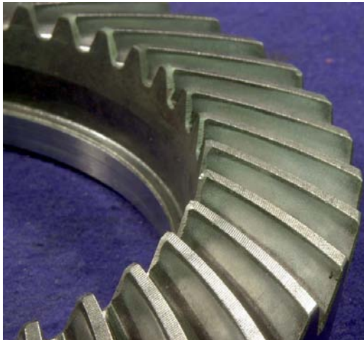
FIGURE 3: ALTERNATIVE VIEW OF RING GEAR TEETH, SHOWING CONTACT PATTERN.
