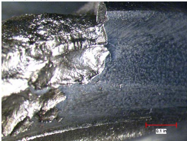
FIGURE 8: PITTING SPALLING FAILURE ON THE LEFT. NOTE AREA OF LOCALIZED HIGH CONTACT STRESS AT BOTTOM OF CONTACT WITH PITTING AT THE TOP.
