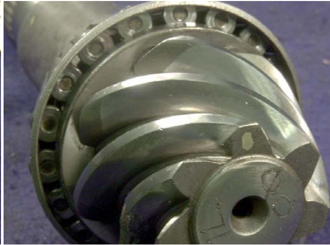
FIGURE 3: ALTERNATIVE VIEW OF PINION SHOWING CONTACT PATTERN.
