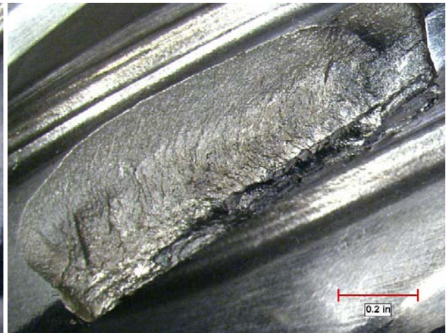
FIGURE 7: CLOSE-UP OF FAILED TOOTH, CONVEX FACE OF TOOTH.
