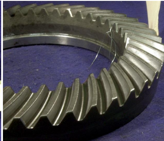
FIGURE 2: RING GEAR TEETH, SHOWING CONTACT PATTERN.
