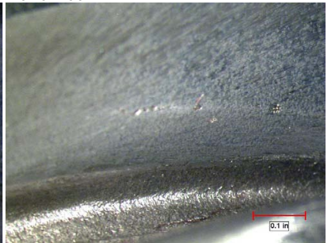
FIGURE 9: AREA OF LOCALIZED HIGH CONTACT STRESS AT THE BOTTOM OF CONTACT WITH LINE OF PITTING AT THE TOP.
