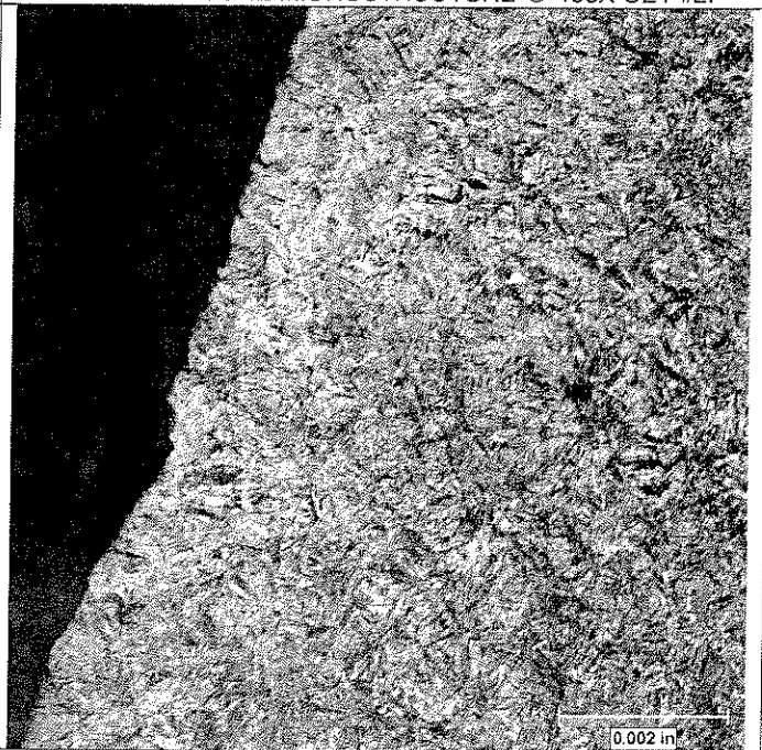
FIGURE 23: PITCH CASE MICROSTRUCTURE @ 400X-SET #3.
