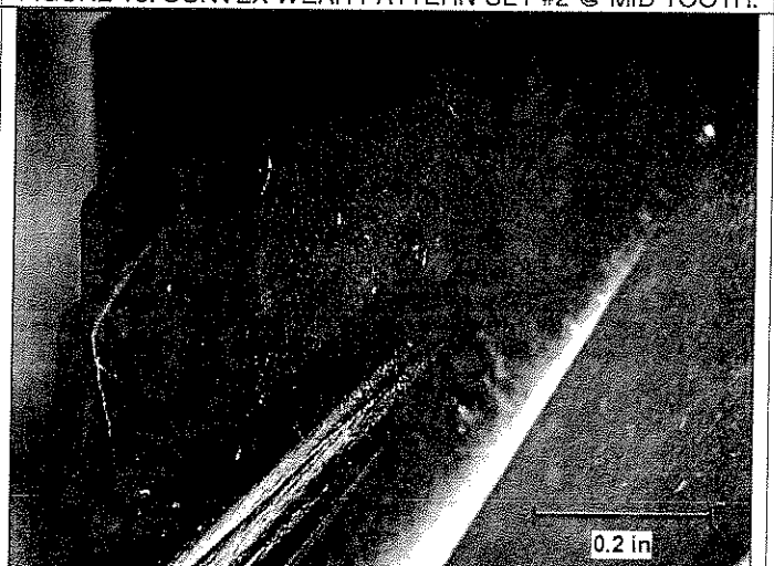
FIGURE 12: CONVEX WEAR PATTERN-SET #3 @ HEEL END.
