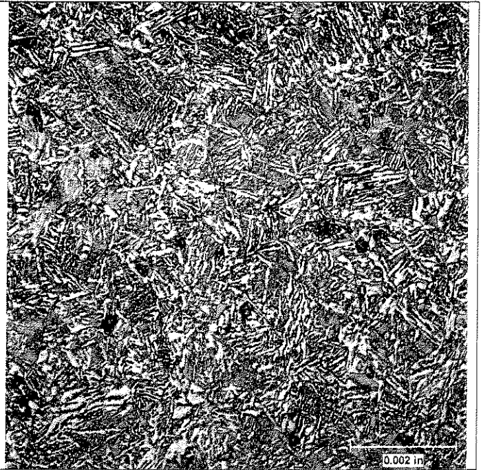
FIGURE 30: CORE MICROSTRUCTURE @ 400X-SET #3.
