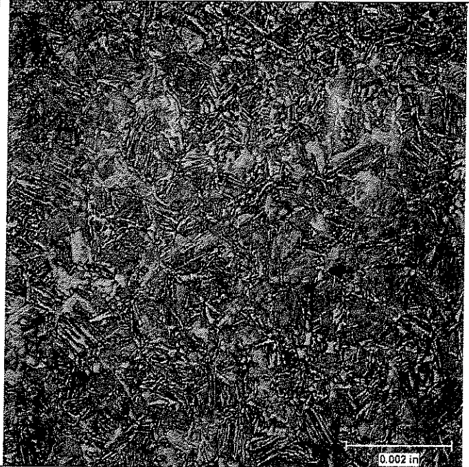
FIGURE 21: CORE MICROSTRUCTURE @ 400X-SET #2.
