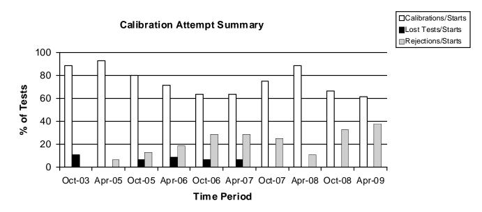
The calibration per start rate has decreased with respect to the previous period. The rejected per start rate has increased with respect to the previous period and the lost test per start rate has remained the same with respect to the previous period.
