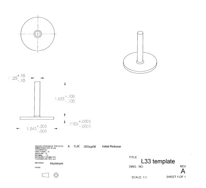
FIG. A1.15 Differential Case, Area 2, Hub I.D. Rating Template
