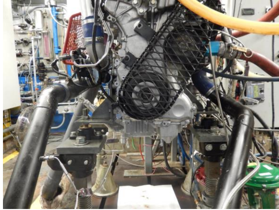
Figure A9.3 Motor mounts, front
