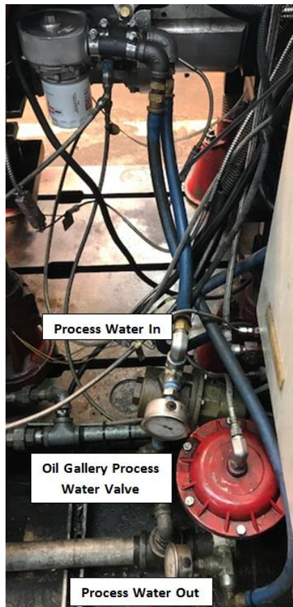
Fig. X Oil Gallery Temperature Control System
