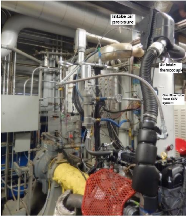
FIG. A9.12 Typical air intake system
