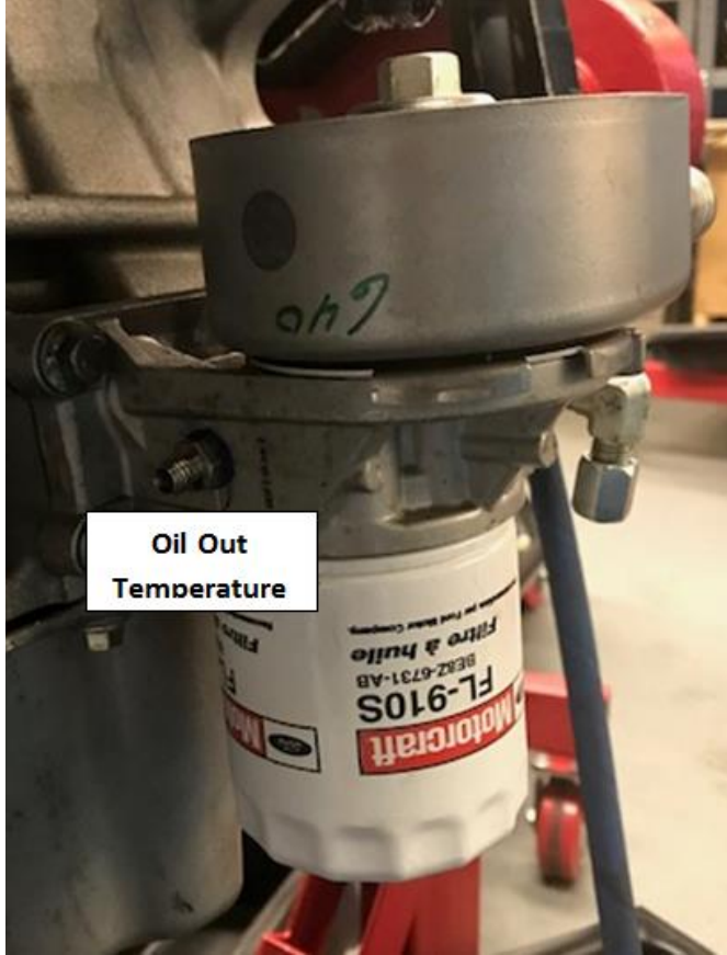
FIG. A9.17 Oil Cooler Showing Oil Out Temperature Measurement Location
