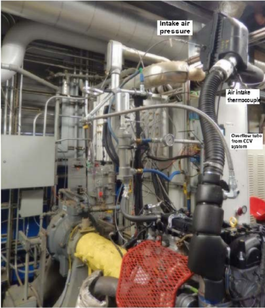
FIG. A2.12 Typical air intake system
