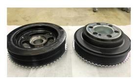
Only the 2016 crankshaft balancer pictured on the right has been approved for Sequence X testing.
