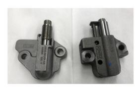
Only the steel tensioners pictured on the right are approved for Sequence X testing. The aluminum tensioners are expected to be approved in the future.
