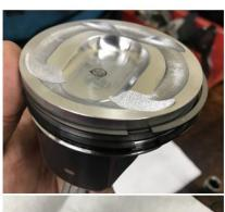
BB and BC pistons have a cast top. AC and AA pistons have a machined top.
