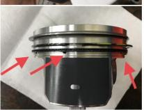
BB and BC pistons have four smoke holes. AC and AA pistons have six smoke holes.
