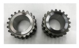
Both gears have been approved for Sequence X testing. The 2018 gear on the left must be introduced on a reference test at each lab.
