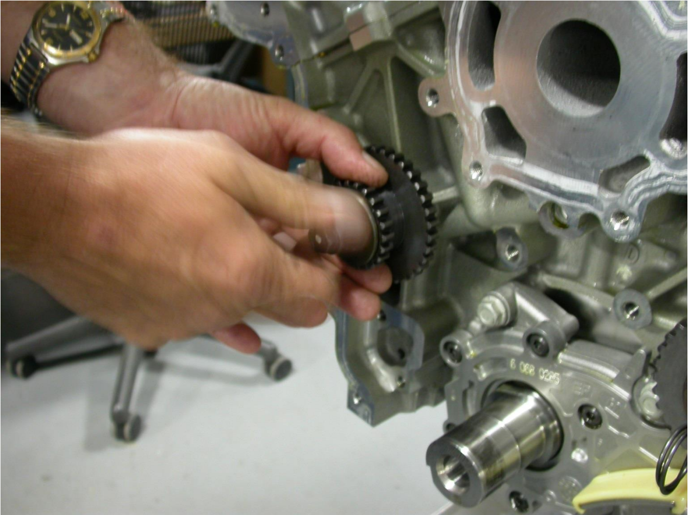
Fig. A17.6 Installation of Right Side Idler Gear
