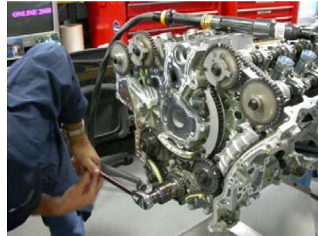
Remove grenade pins from left side idler and tensioners for left side and primary chains.
