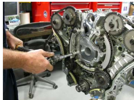
Torque tensioner and chain guides to 23 +/- 3 N·m.
