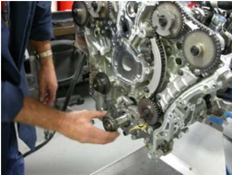
Install right side idler gear and torque to 58 +/- 7 N·m.
