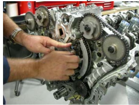
Install left side chain guides.
