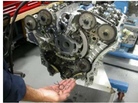
Torque right side idler gear to 58 +/- 7 N·m.
