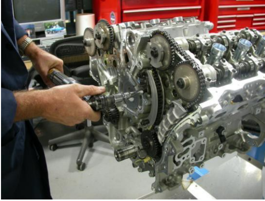
Torque tensioner and chain guide fasteners to 23 +/- 3 N·m.
