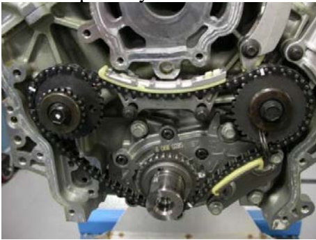
View of primary chain installed.
