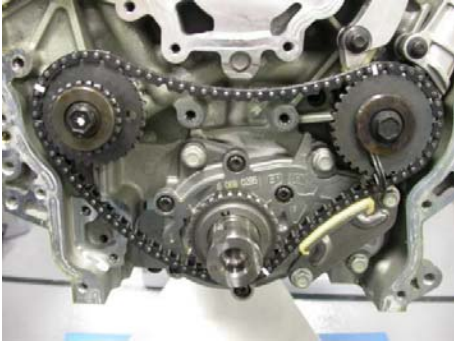
View of primary chain installed.
