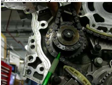
At this point, note hole in right side idler gear as noted by ink pin.
