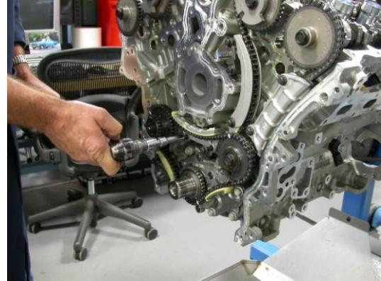
Torque right side idler gear to 58 +/- 7 N·m.
