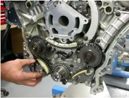
Install primary chain guides.
