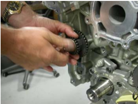
Torque tensioner and chain guide fasteners to 23 +/- 3 N·m.
