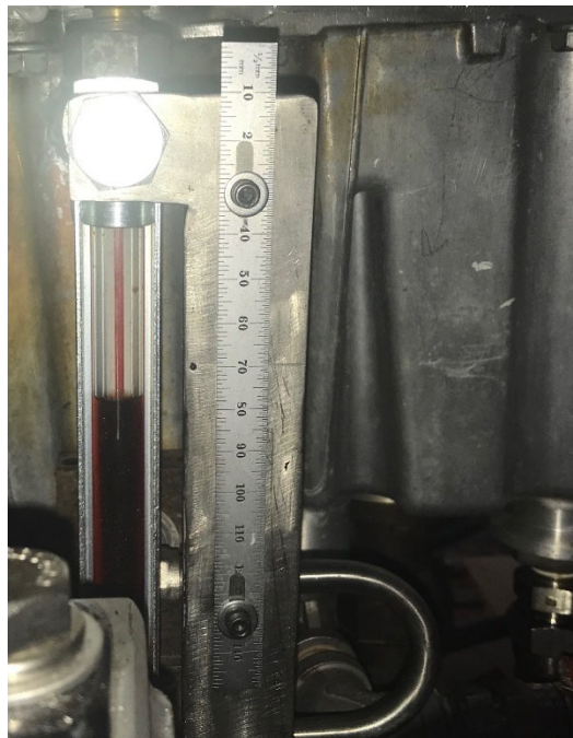
FIG A11.1 Oil Pan Sight Glass Using Metal Attachment with Scale
