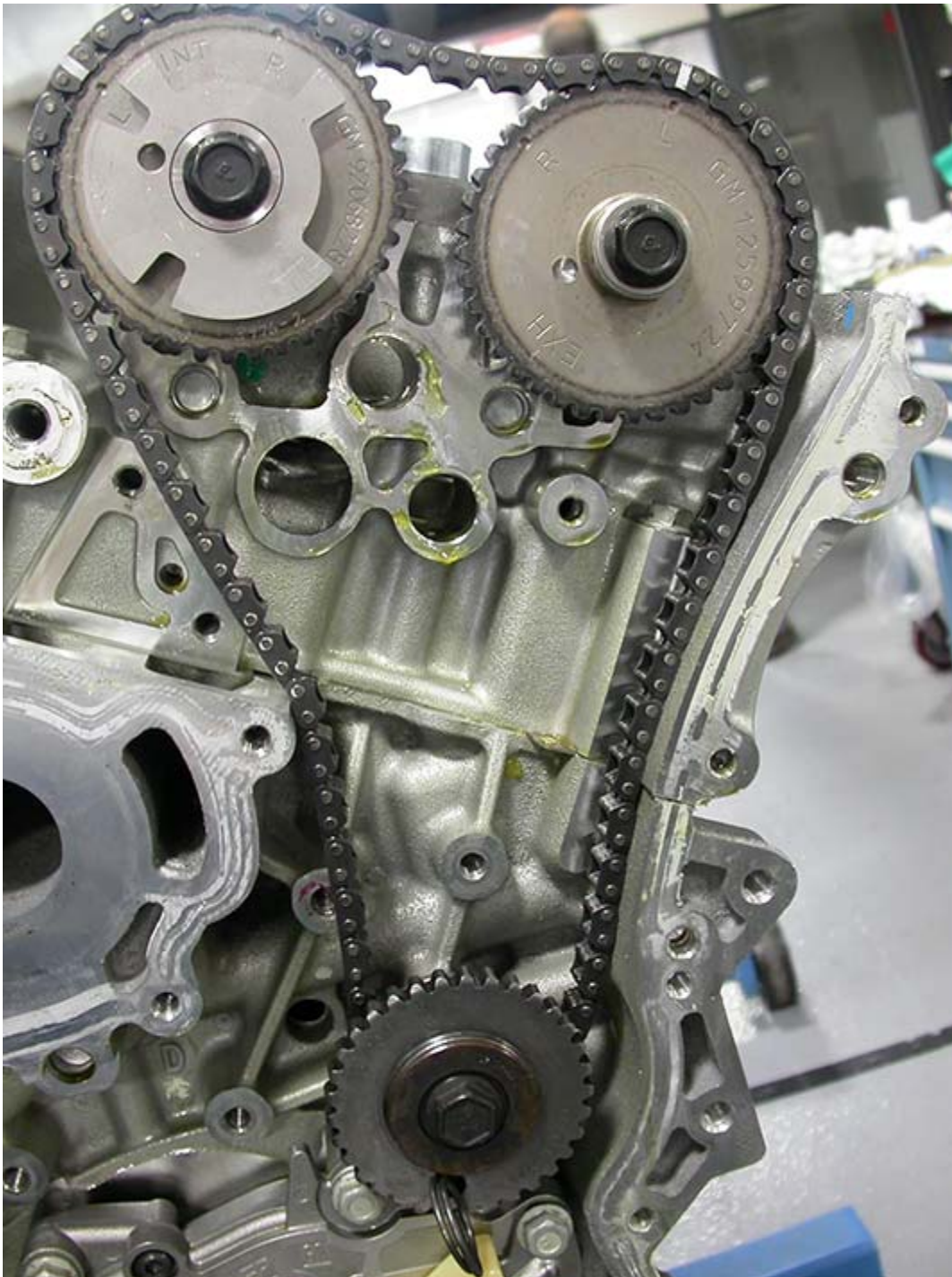
FIG. A17.10 Alignment of Timing Marks, Left Side, with Grenade Pin Installed
