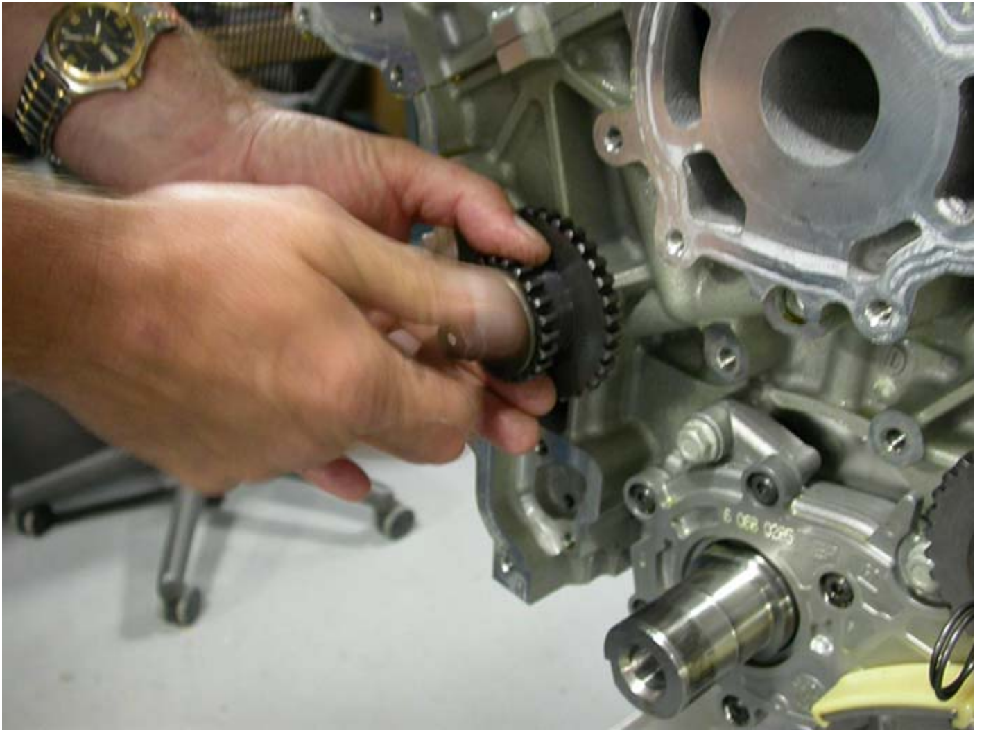
FIG. A17.12 Installation of Right Side Idler Gear
