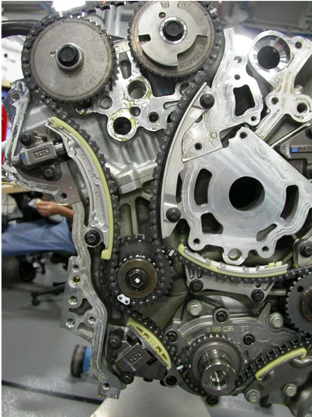
FIG. A17.21 Right Side Chain and Idler Alignment Marks
