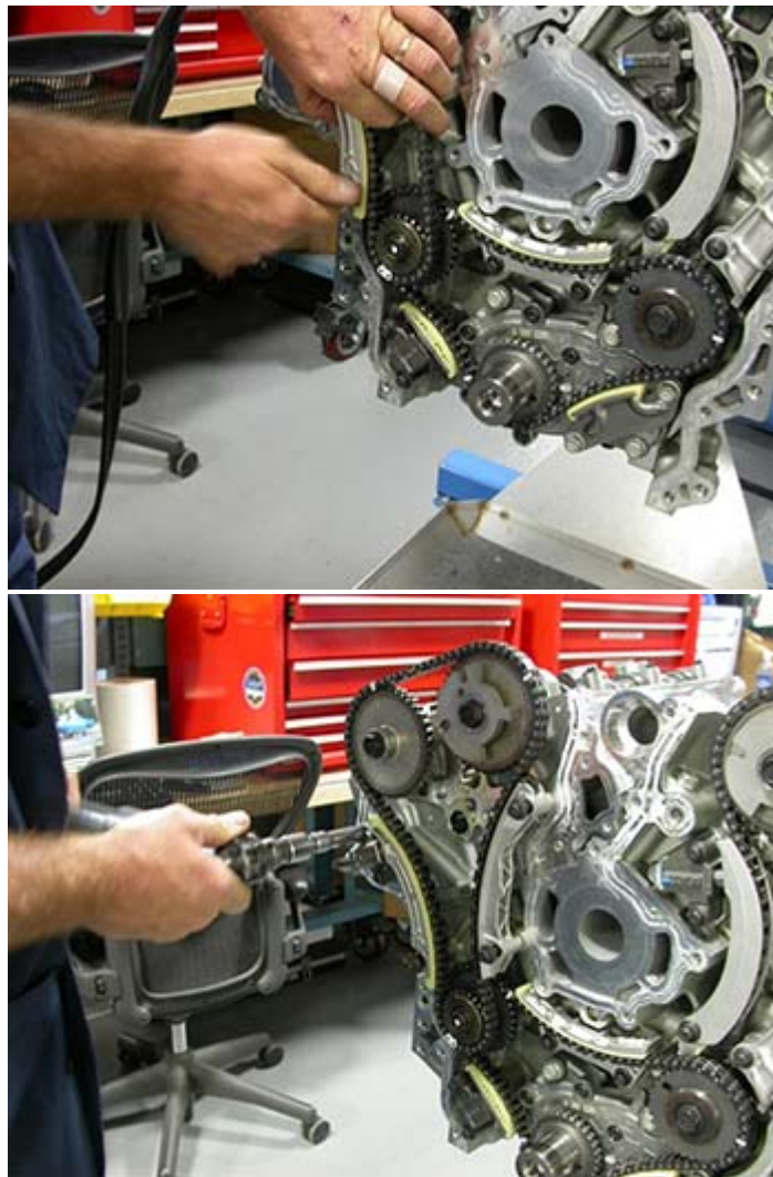
FIG. A17.18 View Showing Chain Guide and Tensioner Installation
