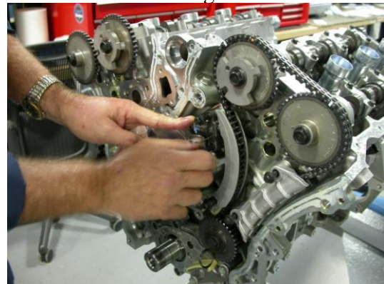
Install left side tensioner and gasket
