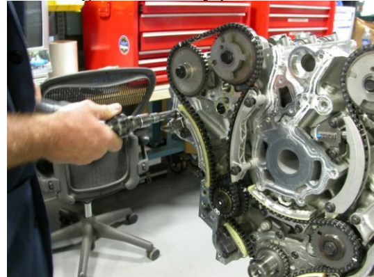
Torque tensioner and chain guides to 23 +/- 3Nm.
