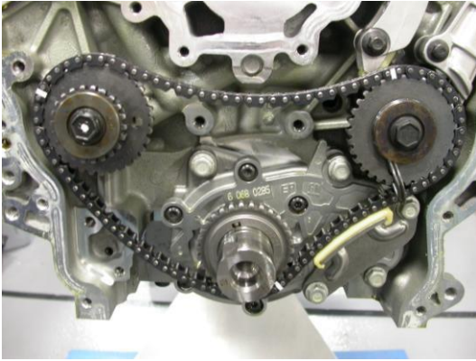
View of primary chain installed.
