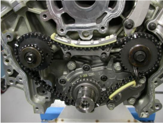
Install primary chain guides.
