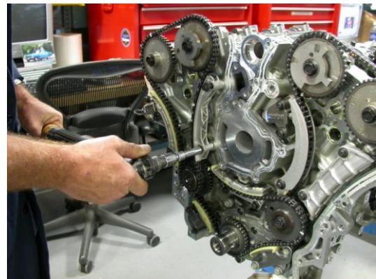
Torque tensioner and chain guides to 23 +/- 3Nm.
