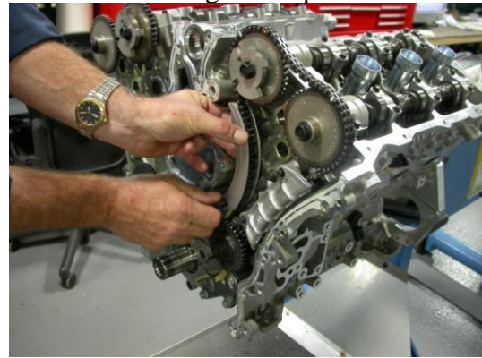
Install left side chain guides.
