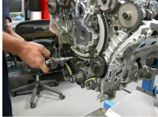
Torque right side idler gear to 58 +/- 7Nm.
