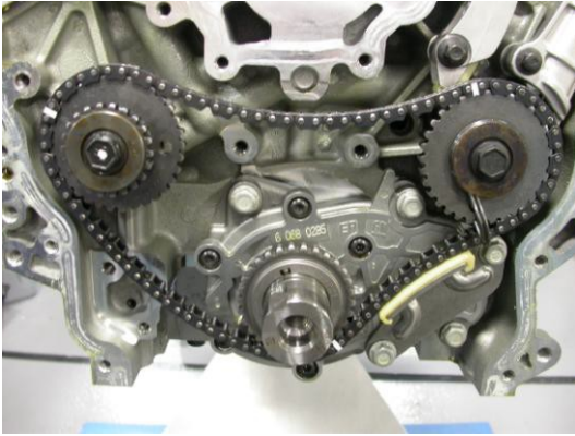
View of primary chain installed.
