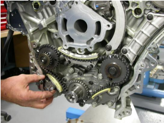
Install primary chain tensioner and gasket. Install tensioner bolt with bushing. Torque tensioner and guide fasteners to 23 +/- 3Nm.
