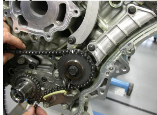
Install primary chain assembly over left, right idlers and crankshaft gears with white identification marks aligned with marks on all three gears.
