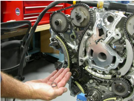
Remove grenade pin from right side chain tensioner.
