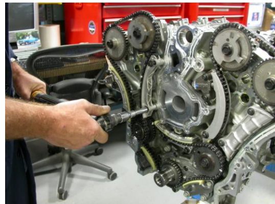
Torque tensioner and chain guides to 23 +/- 3Nm.
