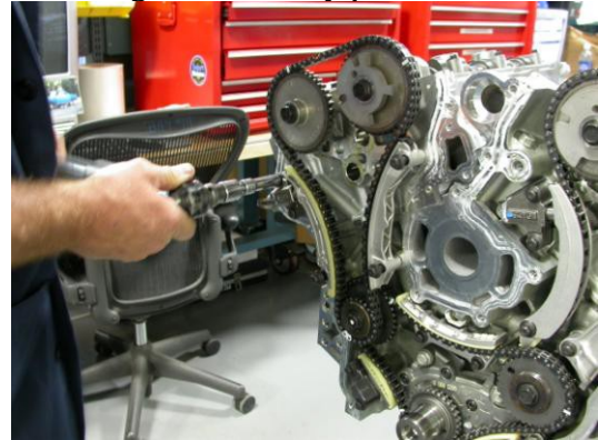
Torque tensioner and chain guides to 23 +/- 3Nm.
