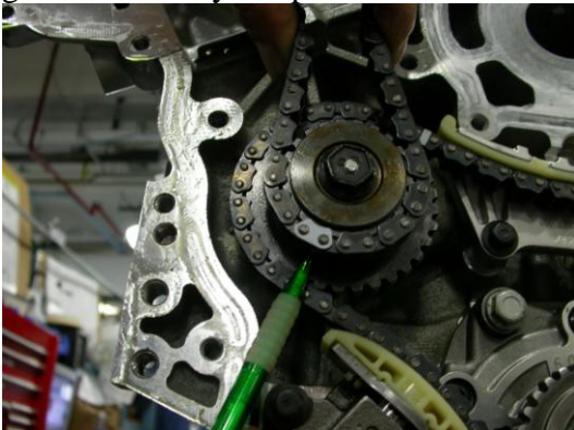
Align right side chain over idler with white link positioned at hole in right side idler and white marks positioned on cam gears at "R" Exhaust and "R" Intake.
