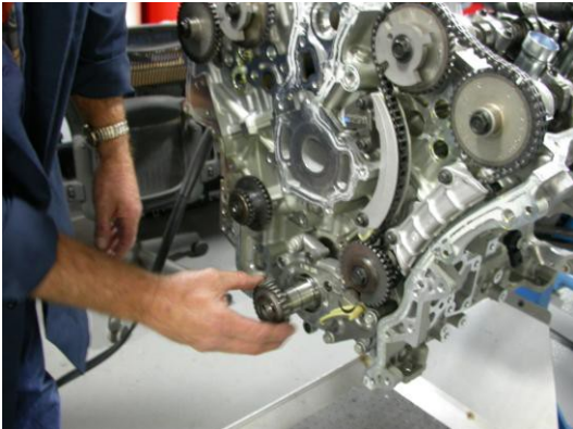
Install crankshaft gear and align dot for left side chain alignment. (Phase 1) alignment step in earlier write up.
