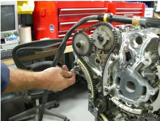
Remove grenade pin from right side chain tensioner.
