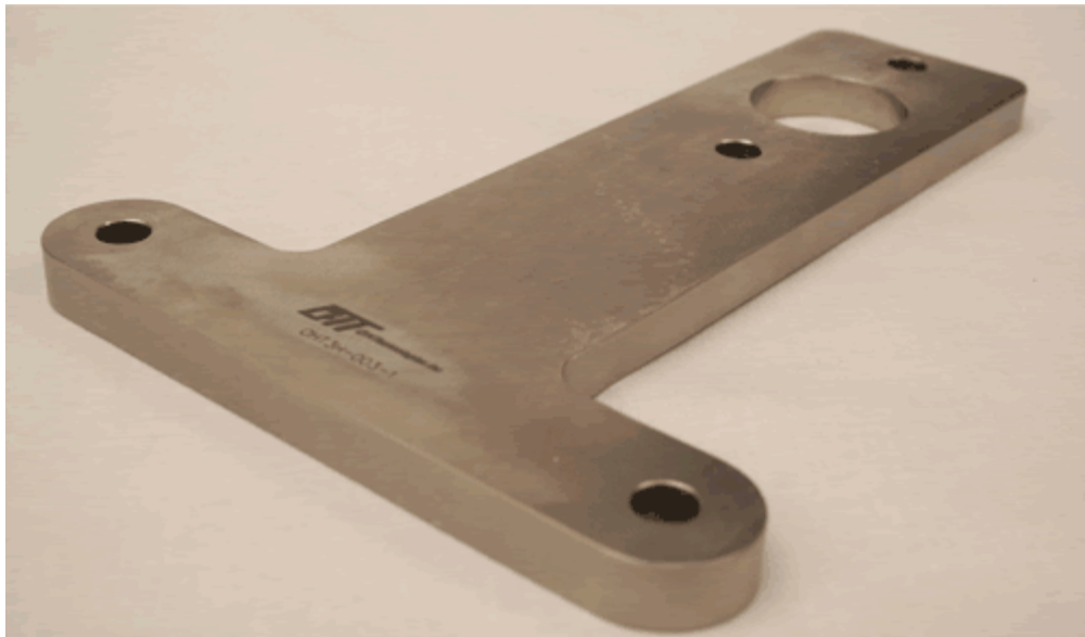
FIG. A5.19 Crankshaft Holding Tool
