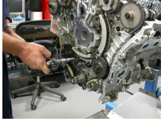
Torque right side idler gear to 58 +/- 7Nm.
