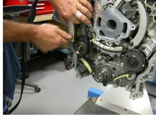
Holding chain together, install chain guides and tensioner. Note, the right bank is the hardest chain to keep tension on during the assembly process.
