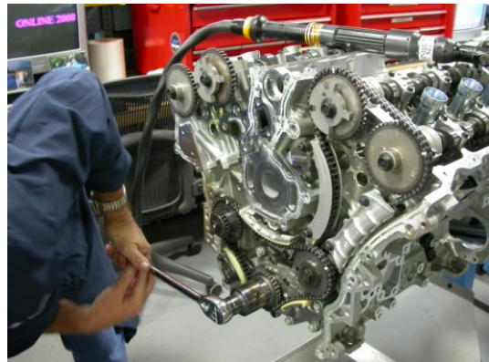
Rotate crankshaft to right side alignment marks. (Phase 2 alignment).
