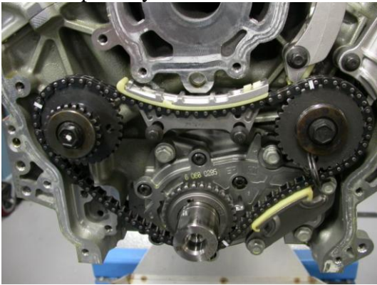
Install primary chain guides.
