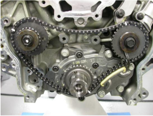
View of primary chain installed.
