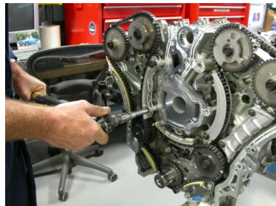
Torque tensioner and chain guides to 23 +/- 3Nm.
