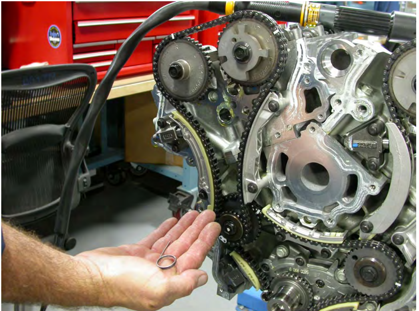
Fig A14.13 View Showing Grenade Pins from Right Side Tensioner Removed
