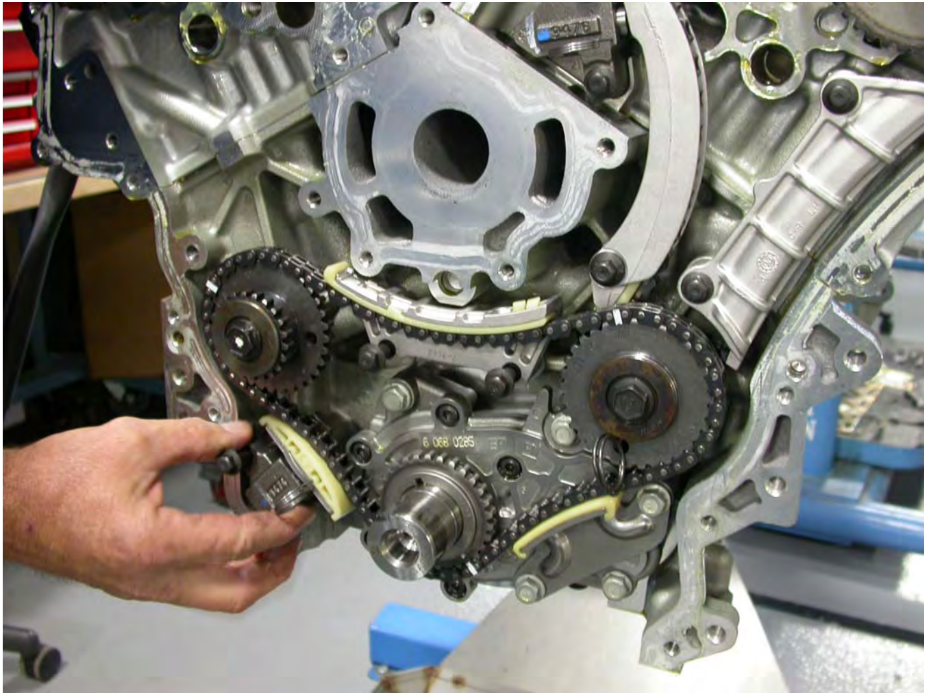
Fig. A14.9 View Showing Installation of Primary Chain Tensioner and Guides
