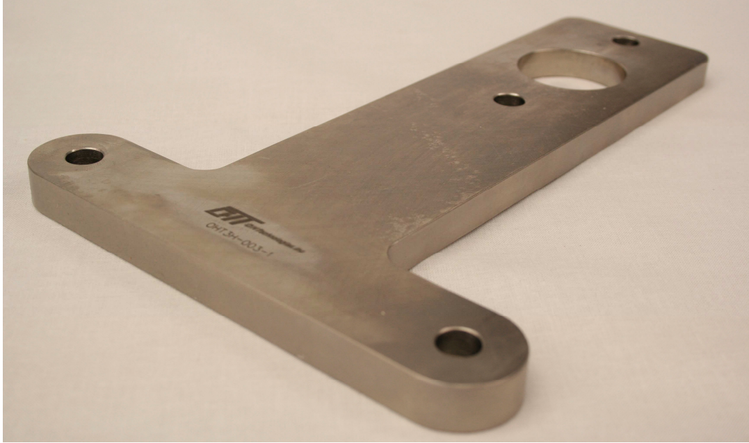
FIG. A2.19 CRANKSHAFT HOLDING TOOL
