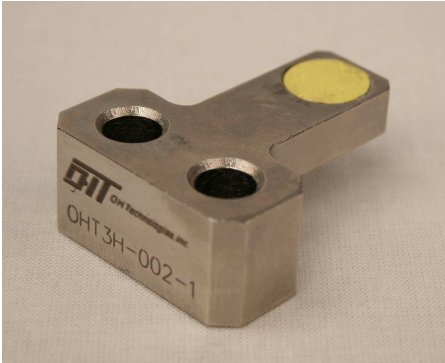
FIG. A2.18 FLYWHEEL TORQUE TOOL
