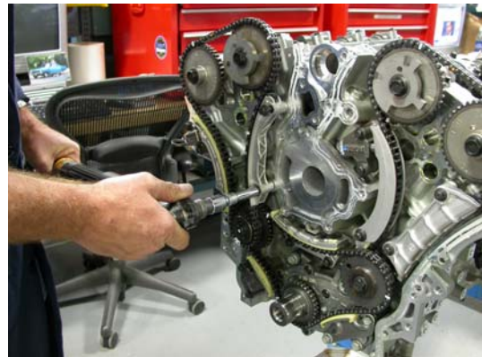
Torque tensioner and chain guides to 23 +/- 3Nm.
