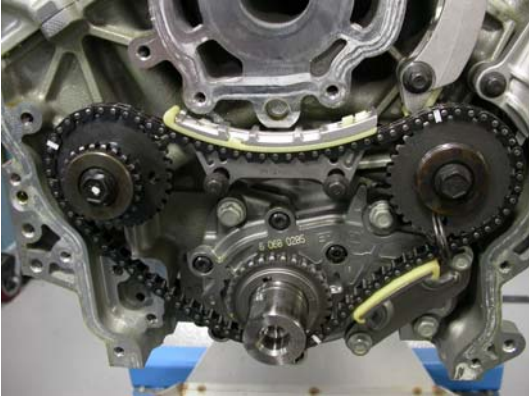
Install primary chain guides.
