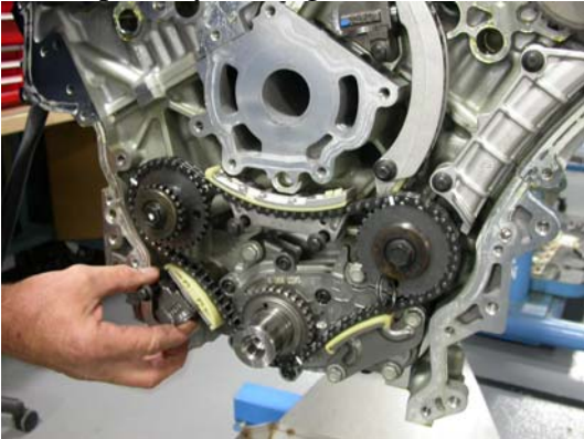
Install primary chain tensioner and gasket. Torque tensioner and guide fasteners to 23 +/- 3Nm.
