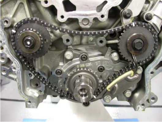
View of primary chain installed.
