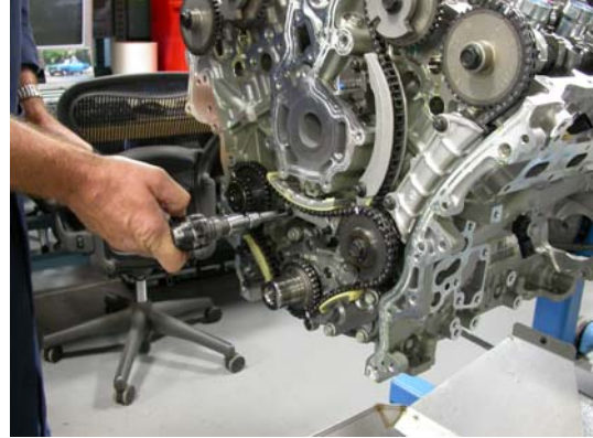
Torque right side idler gear to 58 +/- 7Nm.
