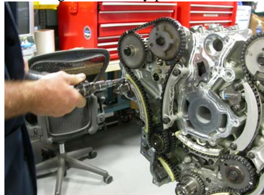
Torque tensioner and chain guides to 23 +/- 3Nm.
