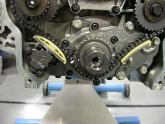
Note white mark on crankshaft gear and alignment mark on oil pump housing.
