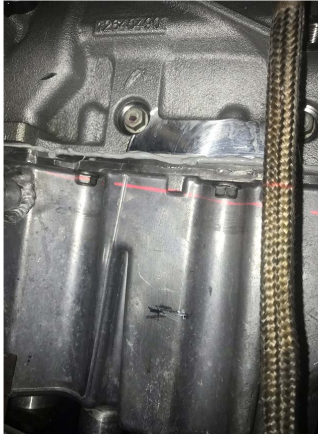
FIG A11.4 Aligning Laser Level with Oil Pan Tab
