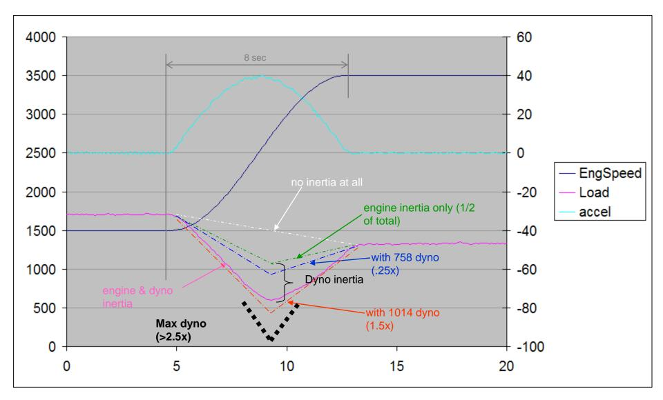
The maximum dyno size that will still provide the same load to the engine is approx 10x bigger than a Midwest 758 (all engine torque channeled into inertia, with no dyno excitation required)
