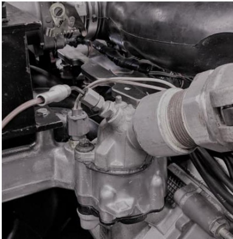
FIG. A7.39 Thermostat Housing with Thermocouple location.
