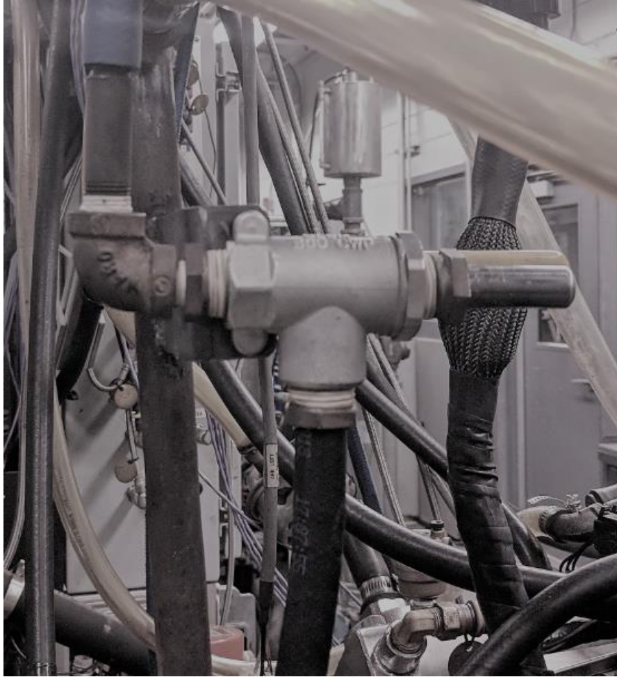
FIG. A7.27 Engine Ventilation System, 3-Way Valve
