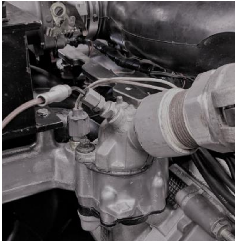
FIG. A7.39 Thermostat Housing with Thermocouple location.
