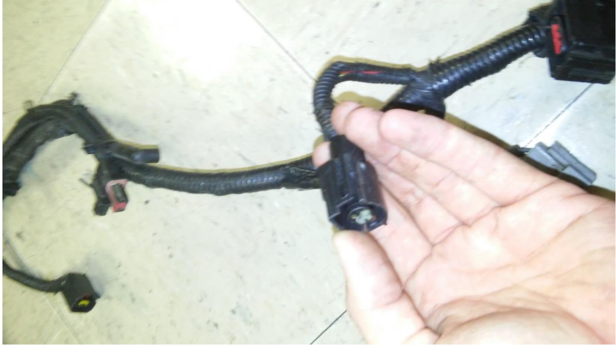
FIG A7.35 Factory coolant temp sensor connector
