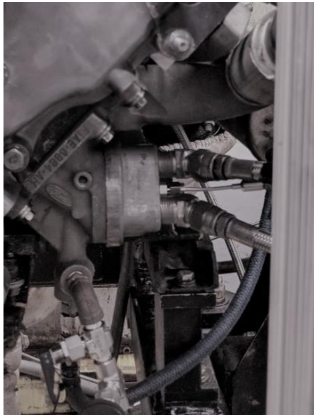
FIG. A7.25 Oil Cooling System, Adapter Housing at the Engine with Typical Fittings for Temperature Sensors, Pressure Tap and Oil Filter
