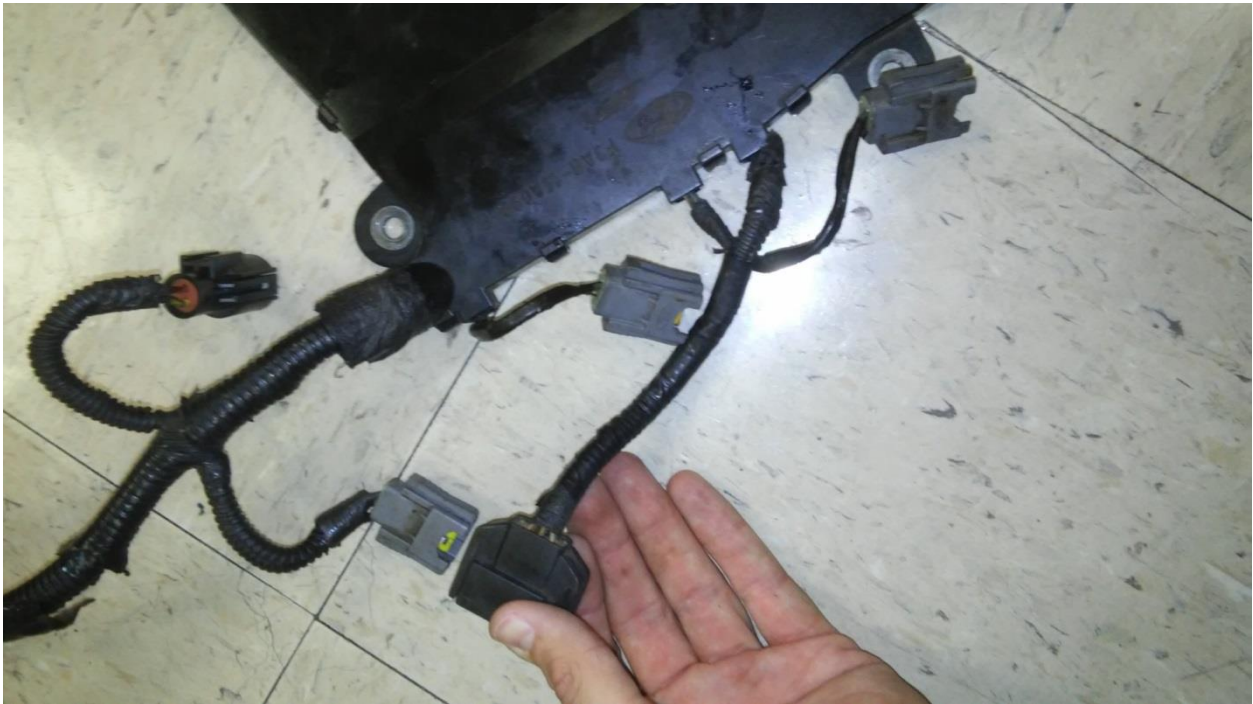
FIG A7.30 Factory throttle position connector
