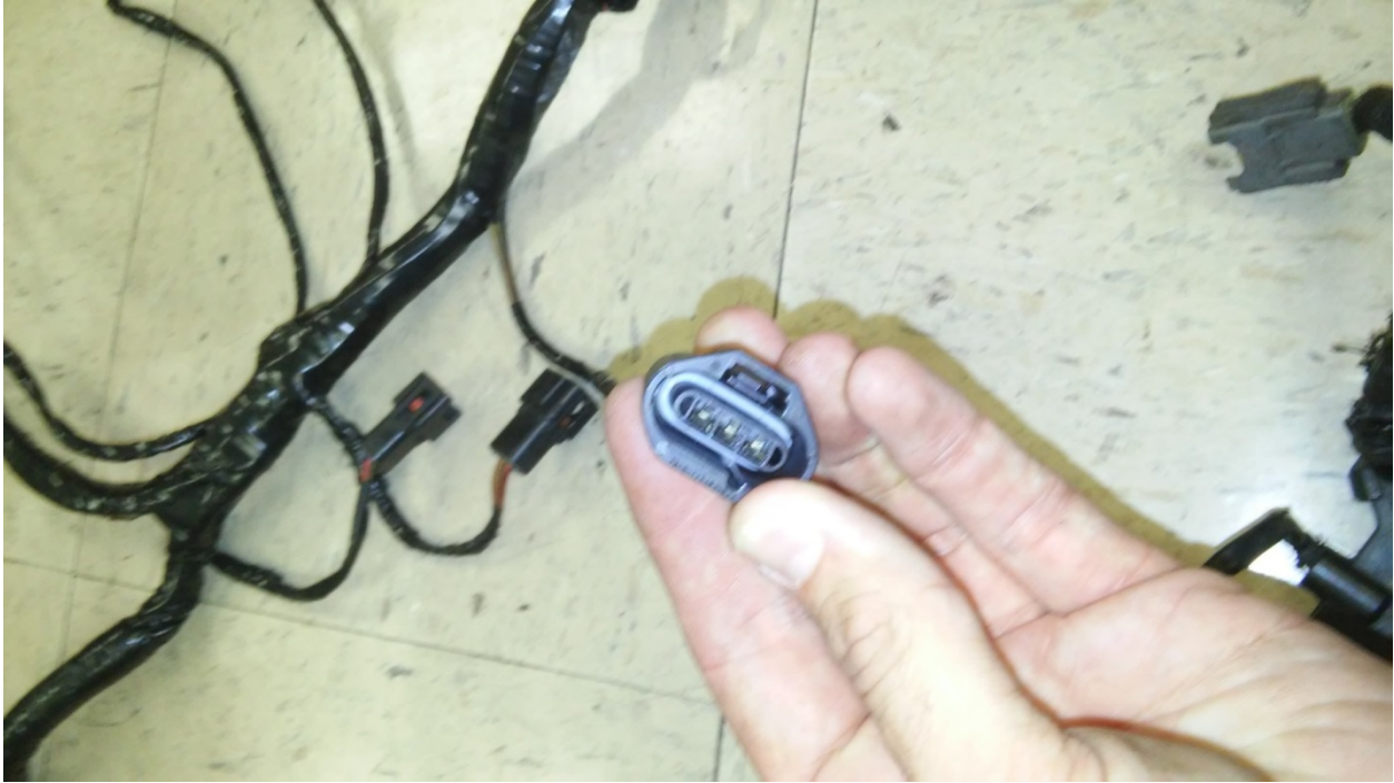
FIG A7.33 Aftermarket (TEI) Throttle Position Sensor connector for 3W7Z-9E926-AA
