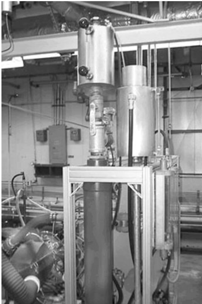
FIG. A7.22 Typical Engine Cooling System
