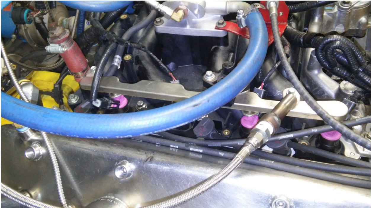
FIG A7.29 Bank one injector wire route without plastic shield
