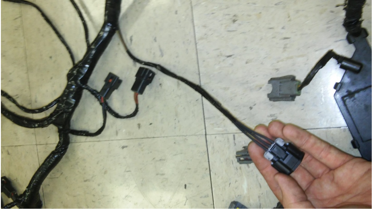
FIG A7.31 Aftermarket (TEI) throttle position connector pigtail installed if 3W7Z-9E926-AA is used
