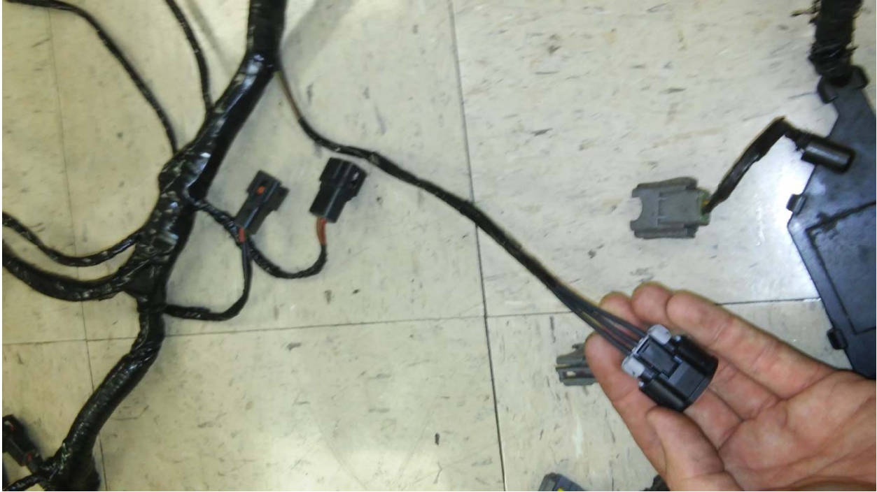
FIG A7.31 New style throttle position connector pigtail installed if 3W7Z-9E926-AA is used
