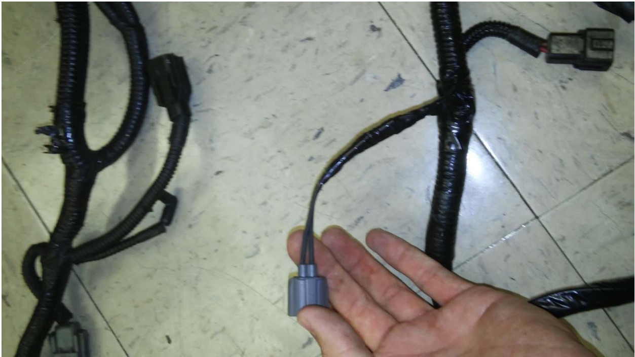
FIG A7.35 New style coolant temp sensor connector pigtail installed.
