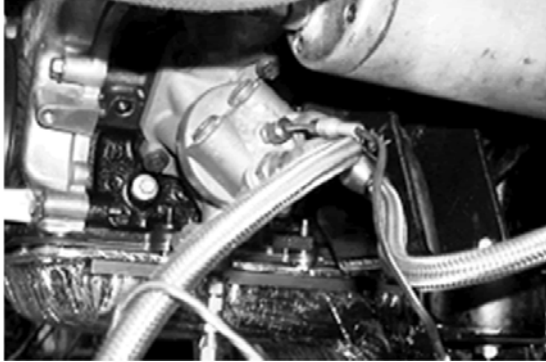
FIG. A7.25 Oil Cooling System, Adapter Housing at the Engine with Typical Fittings for Temperature Sensors, Pressure Tap and Oil Filter
