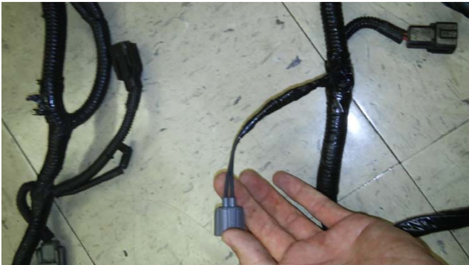
FIG A7.35 New style coolant temp sensor connector pigtail installed.
