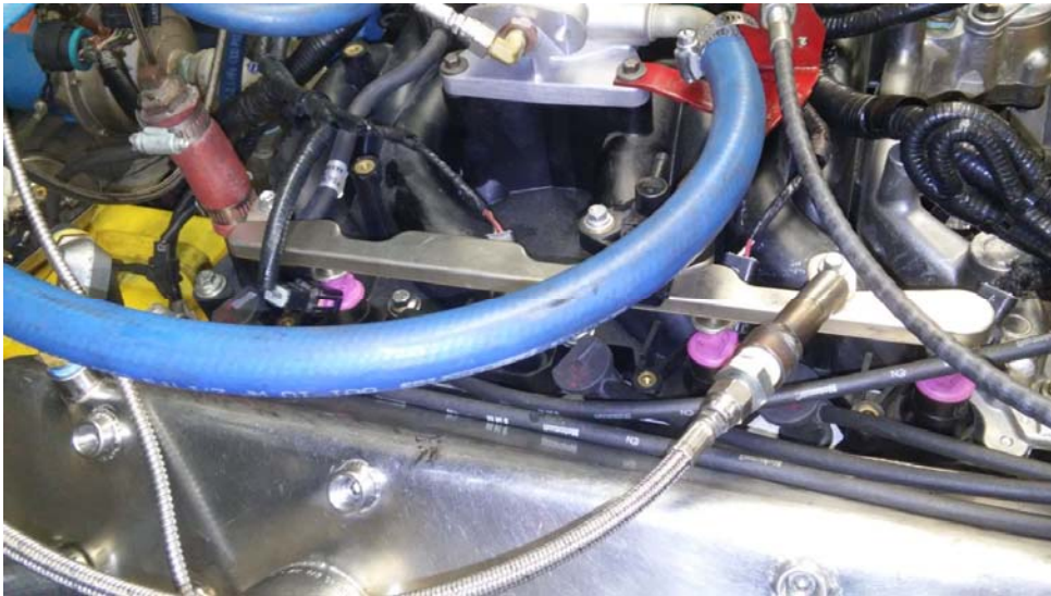
FIG A7.29 Bank one injector wire route without plastic shield
