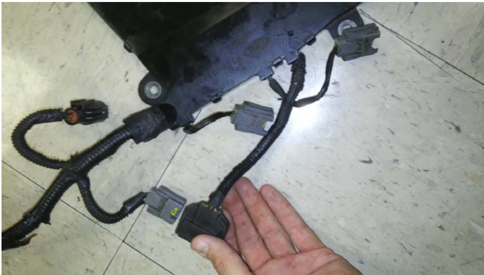
FIG A7.30 Old style throttle position connector
