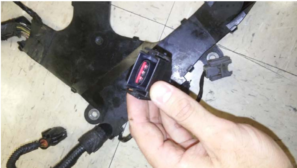
FIG A7.32 Old style Throttle Position Sensor connector for F3PE-9E926-NB
