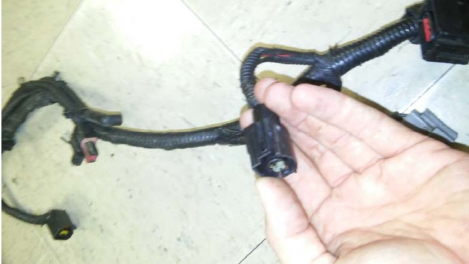
FIG A7.35 Old style coolant temp sensor connector
