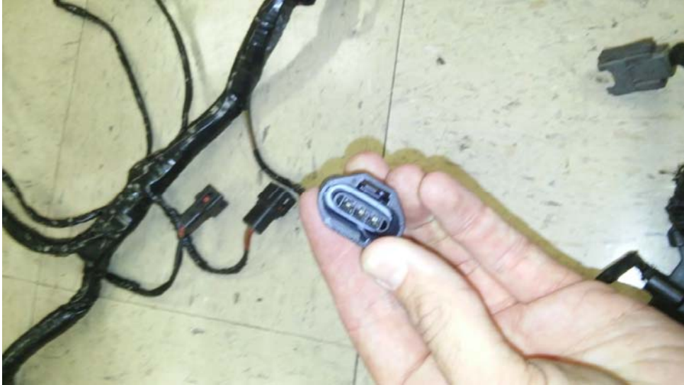
FIG A7.33 New style Throttle Position Sensor connector for 3W7Z-9E926-AA
