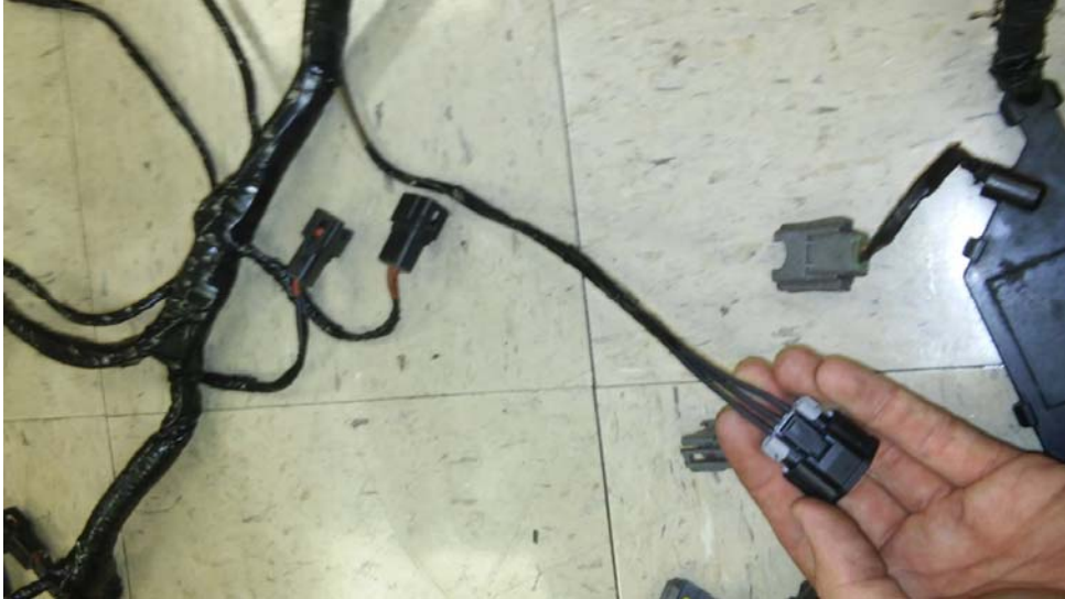
FIG A7.31 New style throttle position connector pigtail installed if 3W7Z-9E926-AA is used
