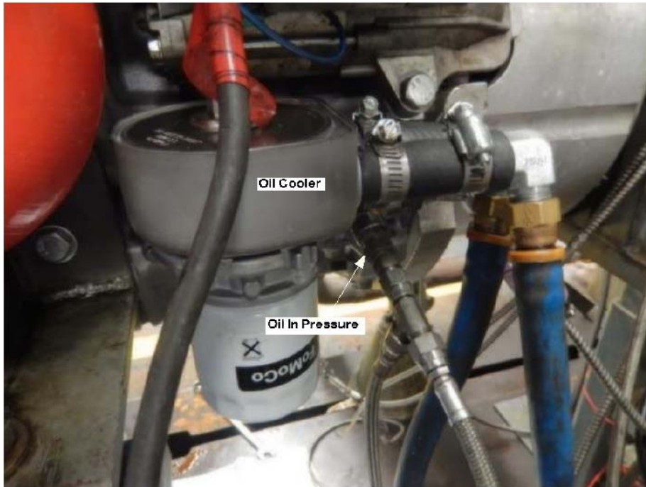
Fig. A6.11 Oil Cooler Showing Oil Gallery Pressure Sensor Location
