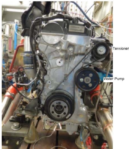
FIG. 3 Water-Pump Drive Arrangement
