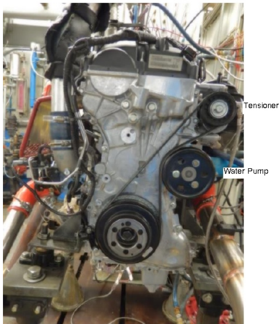
Figure 3 Water Pump Drive Arrangement
