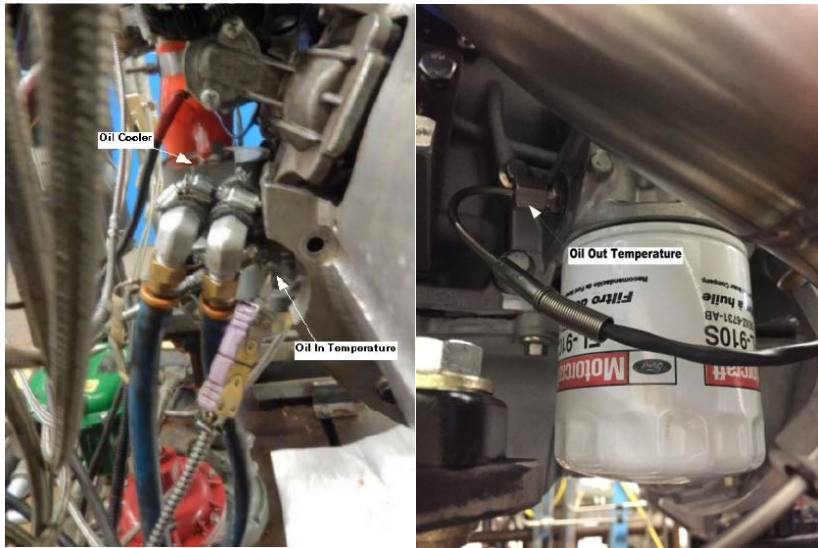
Figure A2.16 Oil cooler showing oil temperature locations
