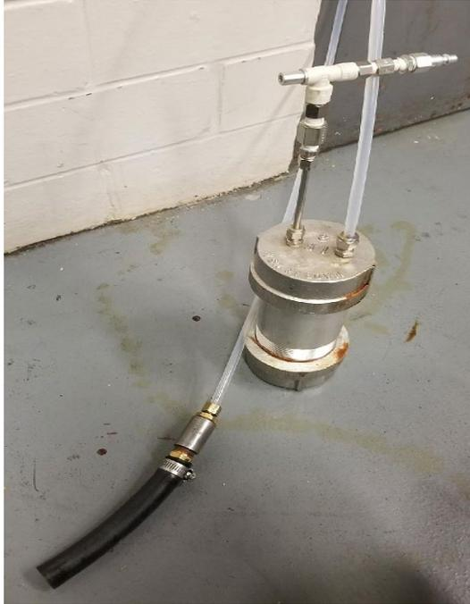
**Fig. X2.29 Vacuum method of oil retrieval canister**
