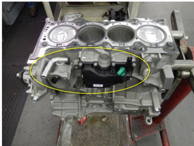
**FIG. X2.13 Cylinder Block Heater Hose Tube and Oil Separator**
