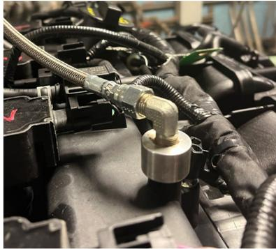
**FIG. X2.20 Crankcase Pressure Connection at Dipstick Tube**
