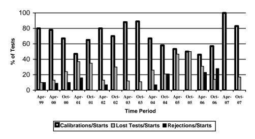
The calibration per start rate has decreased since last period. There were no rejected tests this period. The not for industry statistics not for calibration test was run as a non-blind test to evaluate a new cam batch. This test was run prior to switching to the new cam batch. One test was removed from laboratory and industry control charts due to extremely mild results on the 2005 lot cams. No future testing is planned on these cams in this lab.
