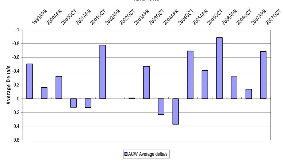
Figure 3 - Sequence IVA Reference Oil Data Average Camshaft Wear
