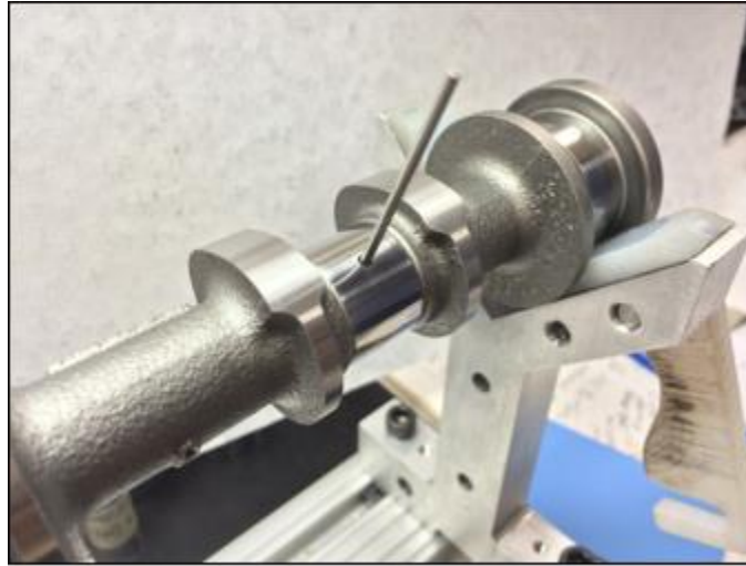
Fig. A5.2 - Measuring Oil Feed Hole Diameters Using a Pin Gage
