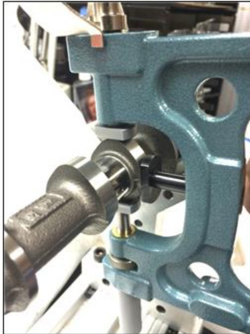
Fig. A5.5 - Positioning the Snap Gage to Measure the Camshaft Heel-to-Toe Height
