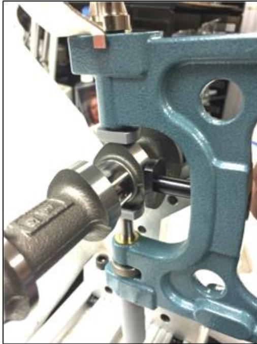
Fig. A5.6 - Positioning the Snap Gage to Measure the Camshaft Heel-to-Toe Height
