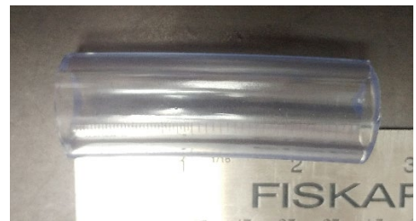
Oil separator top hose, 2 ½ inches long.
