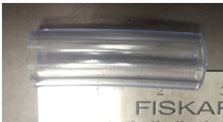
Oil separator bottom hose, 3 inches long.
