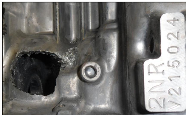
Figure 1 - Photograph of Engine Damage Required for Traceability
