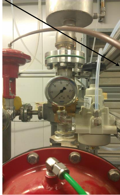
Figure 2 Coolant System Pressure Adjustment
