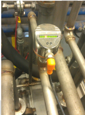
Figure 8. Dynamometer coolant flow indicator
