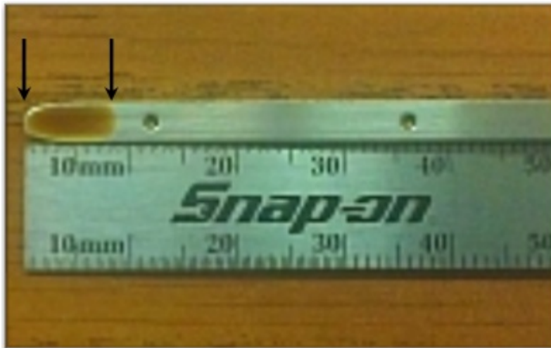
Figure 7: Engine Oil Level Measurement
