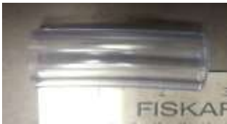
Fig. A8.3 Oil separator bottom hose, 3 in. long.
