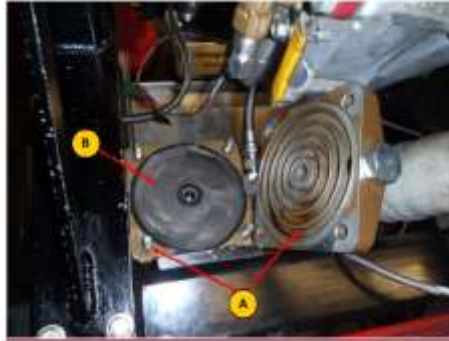
Fig. 2 Disassembled Oberg Filter Housing (A) with filter element (B)
