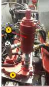
Fig. 9 Oil purge return device (A) connected to the quick connect cap (B)
