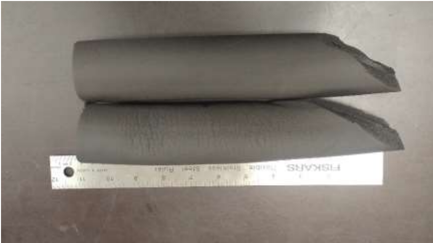
Fig. A8.11 Illustrates the proper cutting of the tubing
