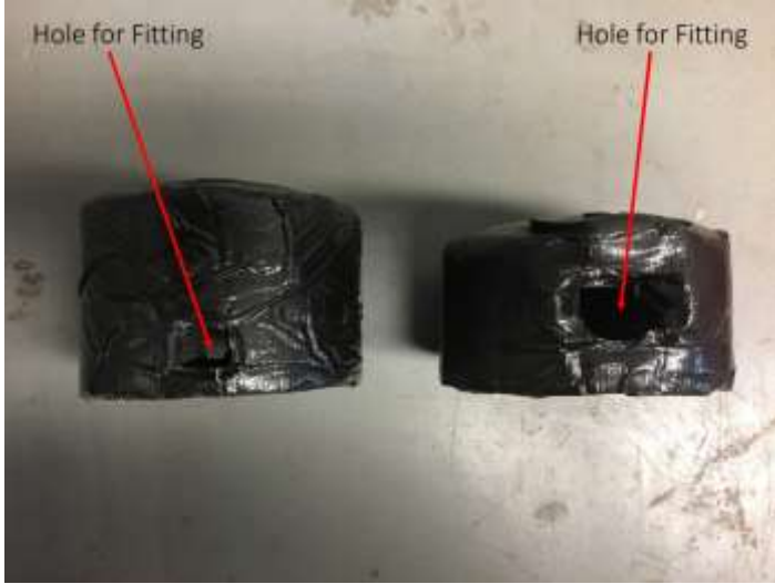
Fig. A8.6 shows the foam wrapping and the hole for fitting.
