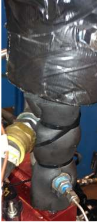
Fig. A8.27 Lower insulation installed with zip ties.
