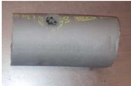
Fig. A8.25 Hole cut for the RAC Gas Out Temperature Thermocouple
