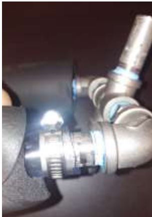
Fig.A8.14 Slide the side insulation to the cross.
