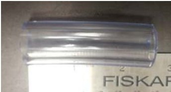
Oil separator top hose, 2 ½ inches long.
