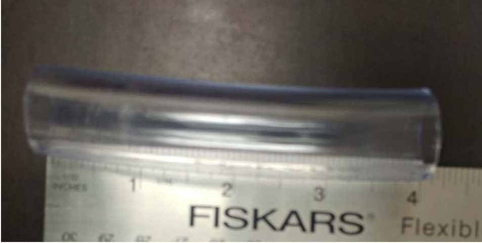
Oil separator side hoses, 2 each, 4 inches long.
