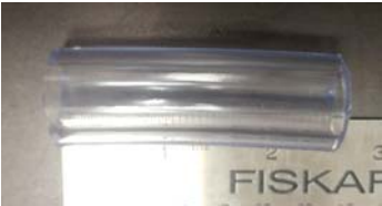
Oil separator bottom hose, 3 inches long.
