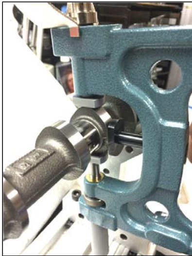
Fig. A5.15 - Positioning the Snap Gage to Measure the Camshaft Heel-to-Toe Height
