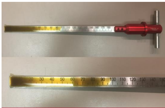
Figure 18. Engine Oil Level Measurement
