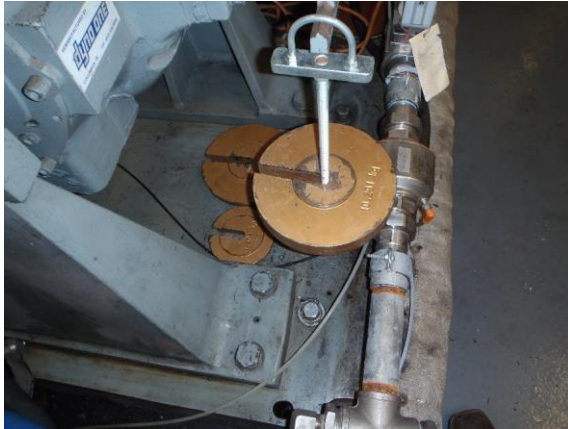
Figure 9. Applying Weights for Dyno Calibration
