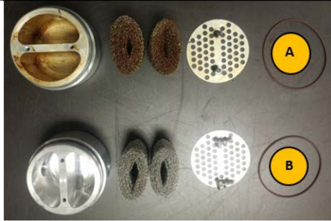
Figure A12.5 O-ring is VITON, dash number 038. 1/16 W x 2 3/4 O.D. X 2 5/8 I.D.
