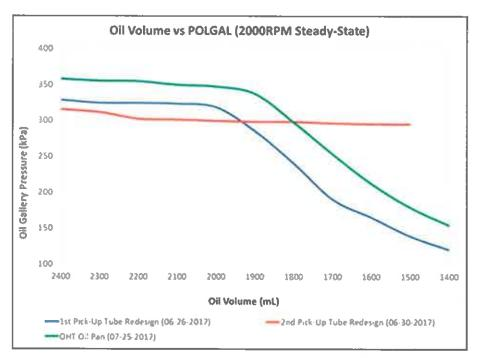
2.2.3.3. The slotted designs (OHT slotted design is shown in right-side chart) do not seem to generate oil pressures that are as good as the oil-well design (shown in left-side chart) under dynamic conditions and extremely low oil volumes.
