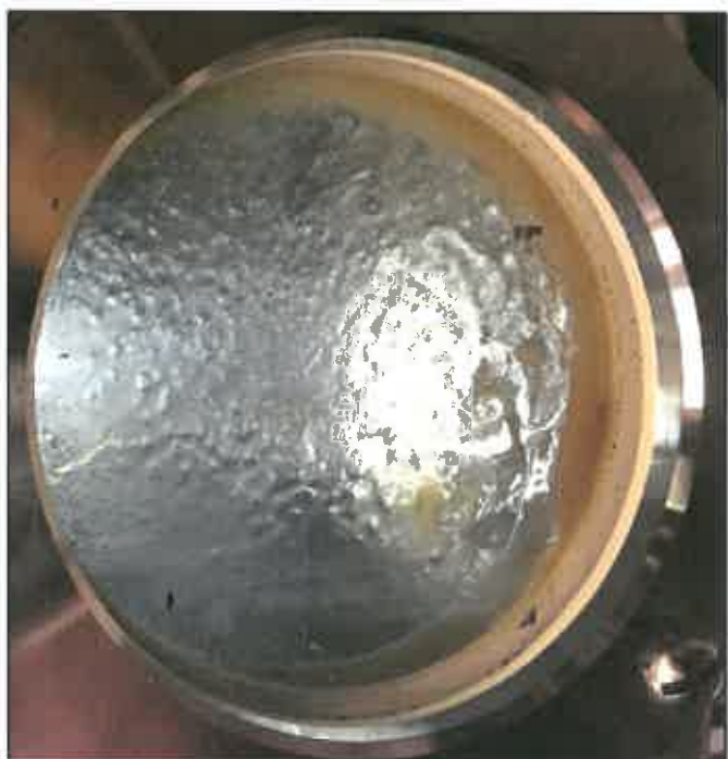
Oil Volume: 2400mL Modified Pick-Up Tube
