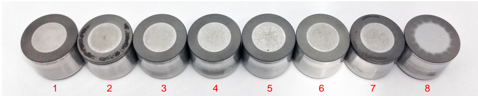
Intake tappets from a failed test
